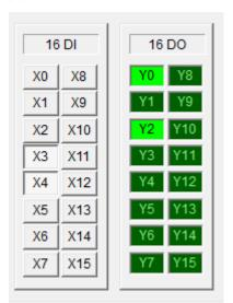
Since the reverse contactor is now de-energized, the reverse auxiliary input(X7) will drop out. Simulate this and turn X7 off. As soon as the PLC sees that the motor is no longer moving down, it energizes Y0. This in turn energizes the forward contactor. The door begins to raise. As per usual, you have 15 seconds to energize the forward auxiliary input(X6). Turn X6 on.
