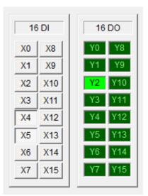
At a certain point, the door will engage the lower limit switch(X3). When you have decided that enough time has passed and that the door should be closed, de-energize X3. Output Y1 shuts off, the reverse starter drops out, and the motor is stopped. The reverse auxiliary input(X7) also drops out. Simulate this by turning X7 off. The door is now closed.
