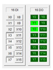
As the door moves down, the upper limit switch(X4) will disengage. Simulate this by energizing X4.
