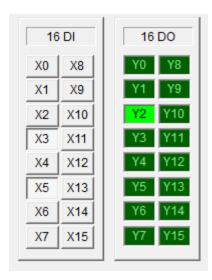
When you feel that enough time has passed that the door should be fully open, engage the upper limit switch(X4) by turning it off. The Y0 output de-energizes and the forward auxiliary input(X6) drops out. Simulate the forward auxiliary input(X6) dropping out by turning X6 off. The inputs and outputs should look the illustration here. The door is now fully up.
