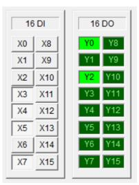
Toggle the wall push button(X0) again. This time the Y0 output will energize, and the door will begin to move back up. Don't forget to energize the forward auxiliary input(X7).
