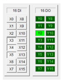
When the door gets to the height you want it to stop, toggle the wall push button(X0). The Y1 output will shut off, killing power to the reverse contactor. Simulate this by turning the reverse auxiliary input(X7) off. Shown here there are no limit switches engaged, the door is halfway opened or halfway closed depending on your outlook
