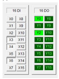
The door is moving up. The kitty cat is safe. Eventually the door will hit the upper limit switch(X4), Y0 will turn off, and the forward auxiliary input(X6) will drop out. Sooner or later the cat will move and the safety photo eye(X5) will input back to the PLC.
